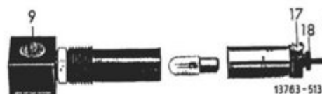
Fig. 11 6 v 15 W lamp attachment 9 dust-glass 17 lamp socket clamping screw 18 lamp centring screw
