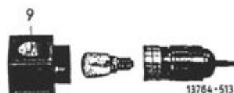
Fig. 10 Micro-dia lamp attachment 9 dust-glass (blue)
