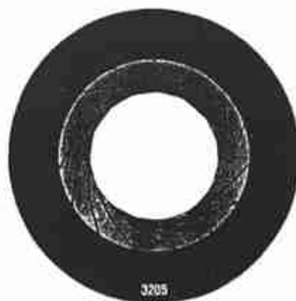
Fig. 5. Appearance of the aperture diaphragm in the objective. It is visible on looking down the tube after eyepiece has been removed.
