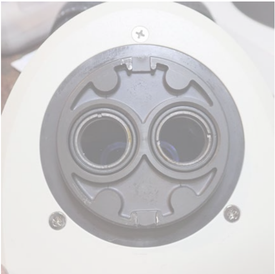
Tubes part 10 455 619 - top section - (eyepiece carrier)
