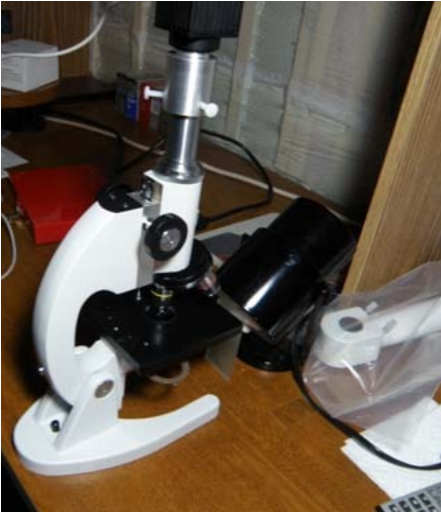
Figure 2: A $20 microscope with standard ISO objectives. This microscope cost as much as the microscope shown in figure 1. For the same price, the image quality is substantially better.
