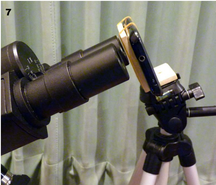
Figures 5-7: Set-up for afocal photography. The correct alignment of the cell phone camera with the eyepiece is important. If the camera to eyepiece distance is not correct, then it is not possible to see an evenly lit image.
