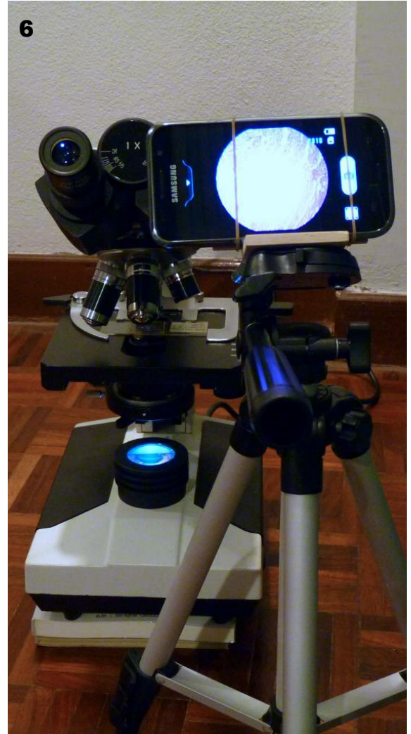
Figures 5-7: Set-up for afocal photography. The correct alignment of the cell phone camera with the eyepiece is important. If the camera to eyepiece distance is not correct, then it is not possible to see an evenly lit image.
