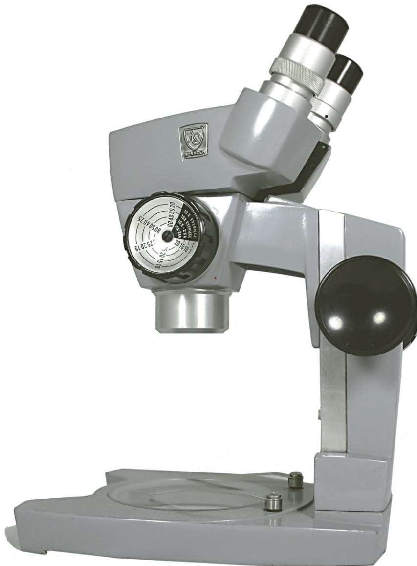
Figure 105 (left): AO Cycloptic model for reflected light, with Magni-Changer "M" (Kreindler, September 2012)
